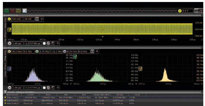
Figure 14. A histogram display plots the relative occurrence of values for the measured parameter, providing insight into the statistical nature of the jitter.
