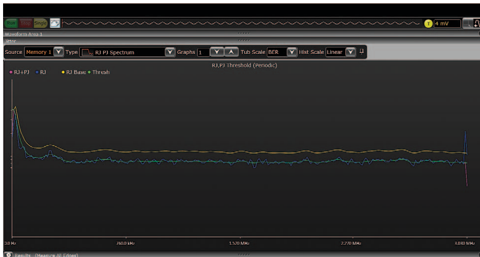
Figure 9. The setup wizard prompts you to select measurement thresholds, histogram, jitter trend, and/or spectrum displays.
