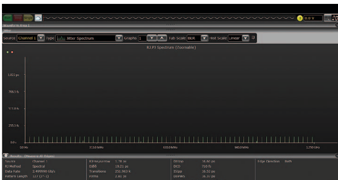
Figure 15. A spectrum display shows the spectral content of the jitter, useful for identifying sources of jitter by their frequency components.
