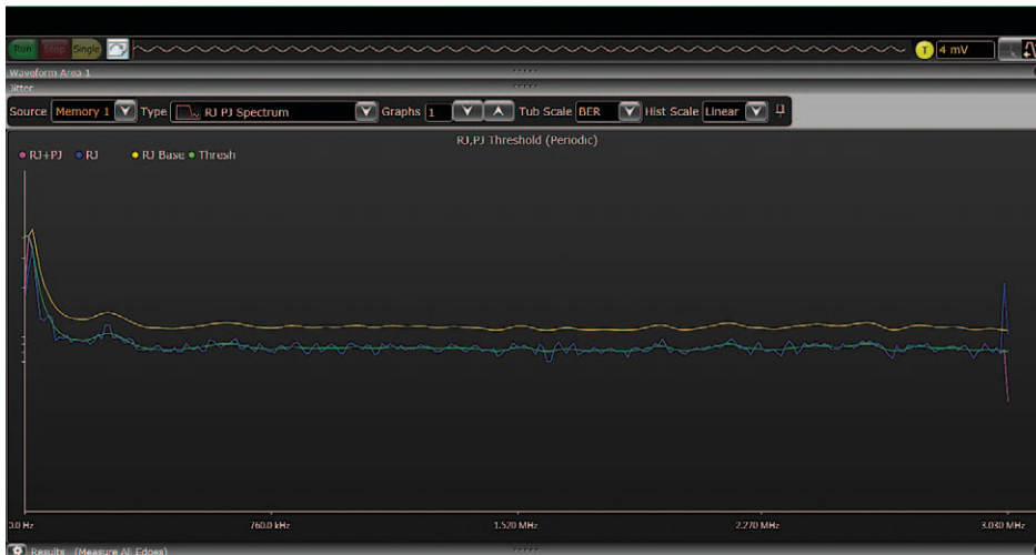
Figure 7. The RJ/PJ threshold allows you to see the exact threshold the software is using to determine RJ/PJ components.
